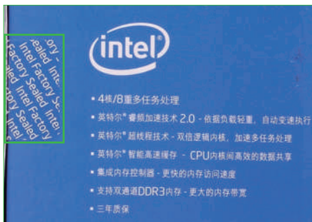
图2-19 Intel CPU的封口标签
